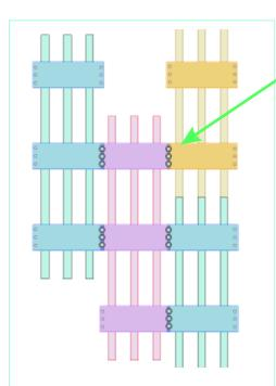
**Figure 3-9** The pre-fab units were staggered to increase strength.
