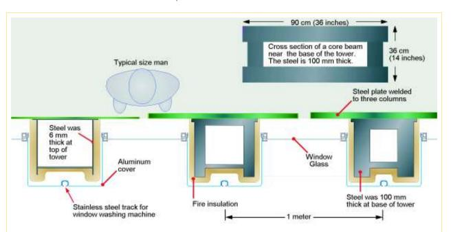
Figure 3-7 Cross section of exterior columns. The steel in each of these three columns is a different thickness to show how the columns varied from the bottom to the top of the tower. The thinnest column would be at the very top of the tower, and thickest would be at the ground. A cross section of the most massive core column is shows for a size comparison. A core column that thick would be at the bottom.
